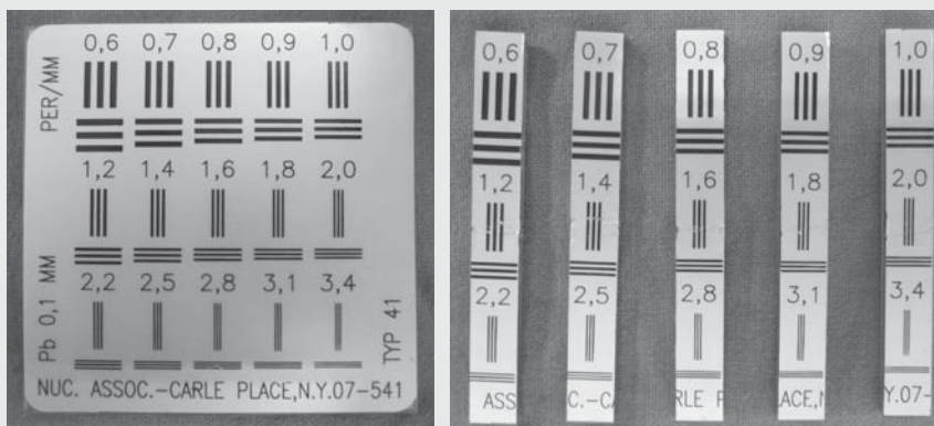
Fig 2. Chosen spatial resolution test phantom. (Left) Nuclear Associates model high precision X-ray test pattern 07-541 (Carle Place, N.Y.) (Right) The test phantom that is laser cut into 5 pieces to make width of each piece to be 6 mm. Laser Cutting was chosen for minimize the possible damage by Mechanical cutting at the 0.1 mm thickness Pb foil which is inside of test phantom.(cited from Choi DH, The image quality assurance in digital panoramic radiographs by using the evaluation table and the phantom stand PhD. thesis, Seoul National University 2012.24)
