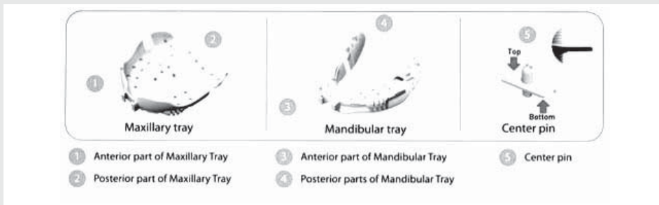
Fig. 1b. Components of DENTCA trays and center pin. The tray consists of two or three pieces, which are detachable, and the center pin is used during gothic arch tracing to find a CR position.
