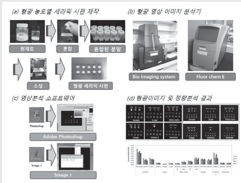
Fig. 3. Whole procedure of the fluorescence characteristics of dental restorative ceramics by using fluorescence digital imaging device.
